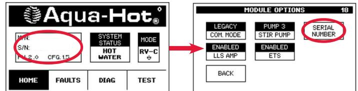
12. Tap "SERIAL NUMBER". The data entry pad will be displayed and here you can enter the serial number shown on the Aqua-Hot Identification label. Tap "ENTER". The Reporter will not accept invalid serial numbers.
