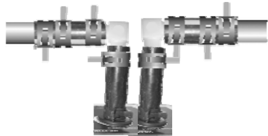
90° Connection Components Installed
