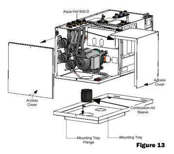
**NOTE:** Remove the bolt securing the front of the access cover to the mounting tray. This bolt will need to be reinstalled once the total installation procedure is complete.
