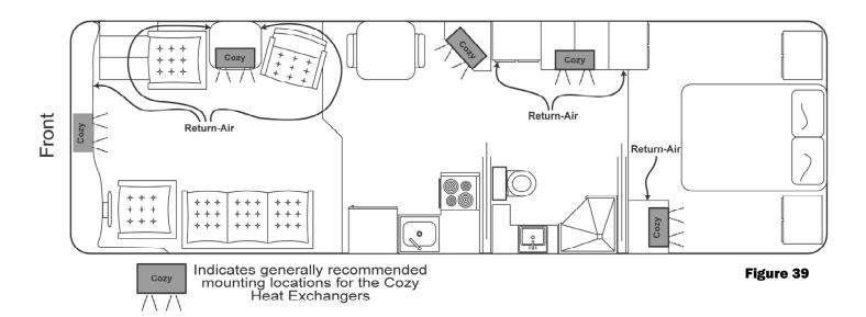
**NOTE:** This is just a sample for mounting locations of the Cozy heat exchangers. Actual placement and quantity may vary on the individual design of the RV. For questions or assistance, contact Aqua-Hot at 574-AIR-XCEL (574-247-9235).
