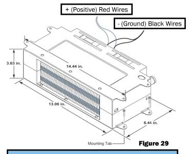
**NOTE:** When wiring the heat exchangers in parallel, the main 18-gauge wire is split to allow the heat exchanger wires to combine with the main wire to be powered or grounded, respectively.
