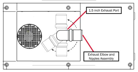
**NOTE:** The exhaust elbow can be rotated 270°, as shown in the illustration; however, the exhaust must not terminate beneath the vehicle or beneath an open-able window or vent.
