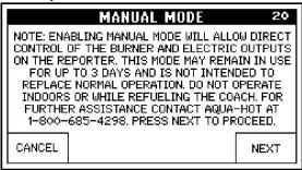
All heating zones are linked together and can be run at 25%, 50%, 75%, and 100% (as shown below). The burner and electric can be enabled or disabled. For all levels, there is a 10 minute duty cycle period that will allow Cozy fans to be on for the specified percentage of 10 minutes. Example, 25% would be on for 2.5 minutes, and then off for 7.5 minutes. It always starts with the on-cycle, then shuts off for the remainder of the 10 minute period.
