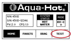
Once the test page is open, select the MANUAL MODE and select "NEXT". Manual mode will continue to run for up to 3 days without any user intervention. Pressing the reset button at any time while enabled will reset the timer, and run for an additional 3 days.
