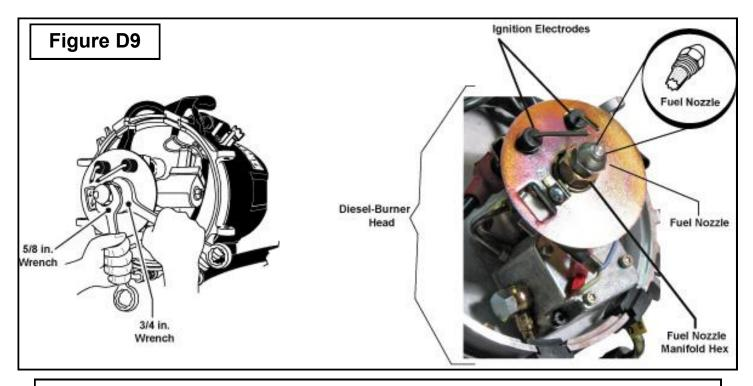
**NOTE:** It is recommended to check fuel pressure any time the fuel nozzle is replace.
