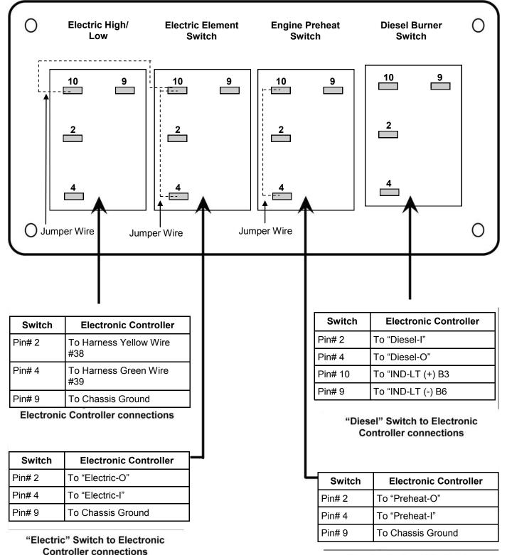
"Engine Preheat" Switch to Electronic Controller connections This section details various components of the Aqua-Hot that may require troubleshooting and/or replacement in the event of a malfunction. The diesel-burner and its components are detailed in Section 9 of this manual.
