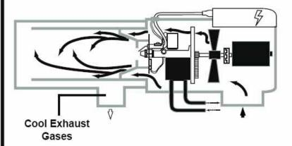
**NOTE:** Whenever the *Diesel-Burner* is switched off by the *VDC/VAC Control Thermostat*, it will automatically be reactivated once the Aqua-Hot Boiler Tank's coolant reaches the preset temperature of approximately 160 (+/-) 5 degrees Fahrenheit.
