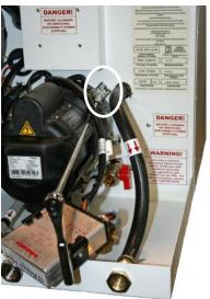
2. The eye-bolt nuts can then be tightened by using a 10mm socket wrench with a 10 inch long extension. Use extreme caution when tightening down the eye-bolt nuts, over tightening of the eye-bolt nuts can cause the aluminum blower casing to crack. (Torque Specifications = Approximately 20-40 in. lbs.)
